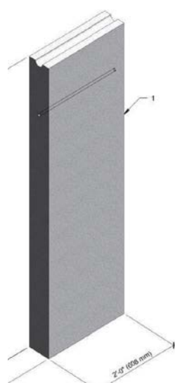
1. AAC WALL PANEL 2. PANEL REINFORCING
